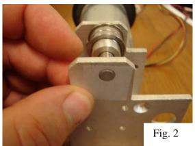
Once the motor bracket is removed from the machine, place a piece of tape over the idler shaft, on the machine side of the motor bracket. This will prevent the shaft from moving during the assembly process, and can stay in place permanently. (Fig 2, above)
