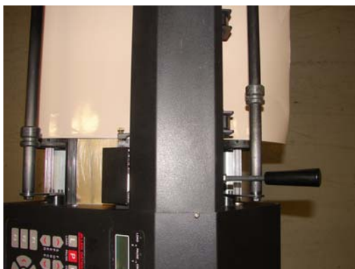
Fig.1 Align material to inside of right sprocket teeth
