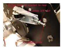
3) Loosen the 3 motor bracket screws using a Phillips screwdriver and 2 set screws in large gold pulley using 5/64 Allen wrench. Slide motor forward to loosen belt on motor. Older machines may have the set screws under the belt, in the teeth of the pulley, which requires the belt to be removed first.
