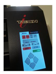
For touchscreen-equipped cutters (serial number ending in 'G'); first enable 'advanced' menus through the following sequence:
