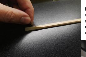
Insert the cut strip in the channel, adhesive side down, starting approximately .5" from the left end of the machine.
