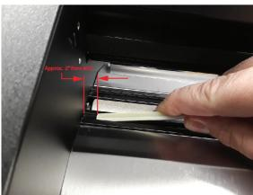
Press the remainder of the strip into the channel, ensuring it is fully seated. Do not run your fingers along the strip, as the corners may be sharp. A screwdriver handle works well for pressing the strip into place.
