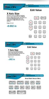
The X and Y Sensor sizes ONLY apply when using multiple marks. Adjusting the X and Y size when using origin only scanning will have no effect on accuracy. When scanning multiple marks, the sensor aproaches the registration marks from multiple directions. The point at which the sensor is tripped may be slightly different from one direction to another. This is where the size adjustment is needed.
