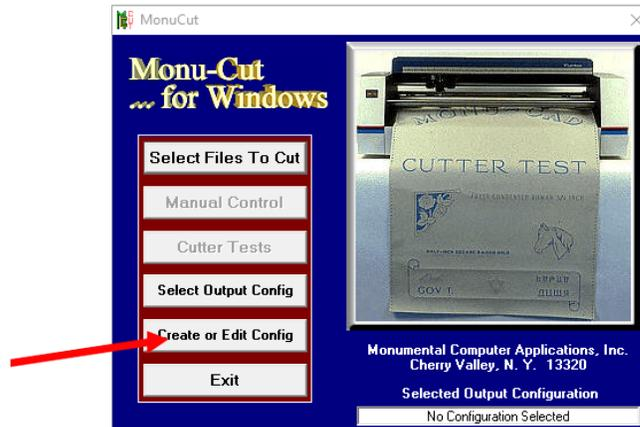
6. In the Configuration screen, different settings should be set according to the type of cutter connected to the PC. For this example, an Allen Datagraph cutter with graphic panel will be configured. It is important to note that MonuCut does NOT support Ethernet connections. USB/serial connections are supported for cutting.
