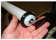
3) Reinsert the axle to the dancer arm, making sure that you align the flat on the shaft with the set screws.
