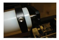
2) Slide dancer bar to left to disengage from arms. Slide both infeed guides onto the white dancer roller.
